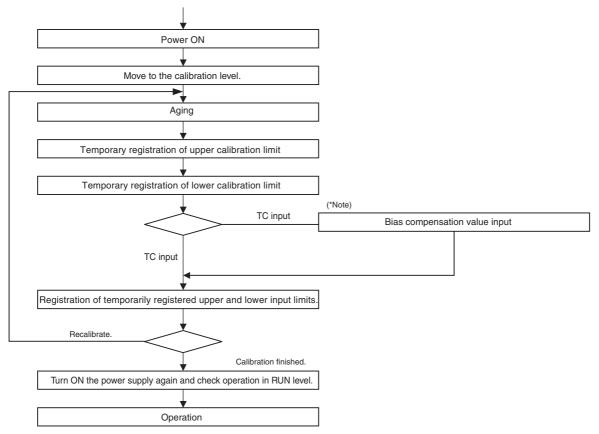
\* The previous calibration value is not displayed when the status of bias compensation values is being monitored. The display cannot handle bias compensation values because they are temperature readings rather than a count. This means the value that is read during calibration is not a bias value, but the calibration value for the main input.
