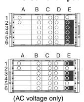
Input the signal to be measured. The following figure shows the inputs that can be measured by each model. Connect the input devices to the terminals shown below according to the input type.
