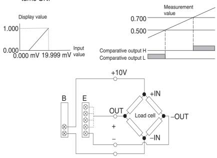
\* 2 mV/V indicates a load cell output of 2 mV for 1 V applied voltage for the rated load (when using a load of 1 N). When the applied voltage is 10 V, the load cell output is 20 mV (2 mV×10)
