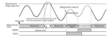
The PV display will show "----" during RESET input (no measurement status).
