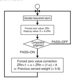
Application Example: Absorbing temperature drift for linear sensors
