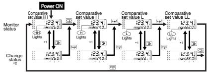
\*1 If no key is pressed for 5 seconds, the set value is registered and the display returns to monitor status.
