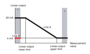
\* If the upper and lower limit are set to the same value, then the upper limit will equals the lower limit plus 1 for linear output.
