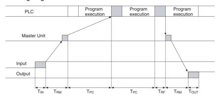
T<sub>IN</sub>: ON/OFF delay time of the input slave (0 used as minimum value)
