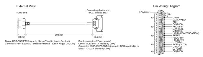
**Note** D-sub connectors are connected to the BCD output cable.
