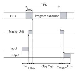
T<sub>IN</sub>: ON/OFF delay time of the input slave (0 used as minimum value)
