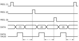
\*Maintain a 20 ms interval from when DATA VALID turns OFF to the next REQ signal.
