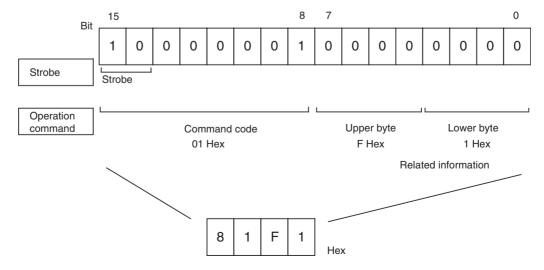
With the CS1W-DRM21 and CJ1W-DRM21 DeviceNet Units, operation commands are made ready for execution by writing to the allocated words (CIO 3202 when the default I/O allocation (fixed allocation area 1) is set.)
